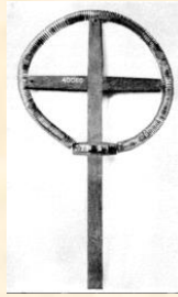
One of Hertz's radio wave receivers: a loop antenna with an adjustable micrometer spark gap
